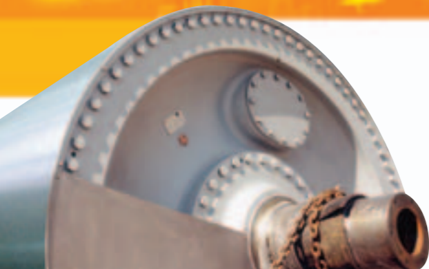
Presse chaude revêtue - Ø2500mmx4300mm - poids: 25 tonnes Ø2500mm x 4300mm - 25MT - coated hot press
