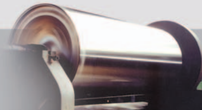
Rectification d'un cylindre sécheur - Ø1500mmx3000mm Grinding of a Ø1500mm x 3000mm drying cylinder
