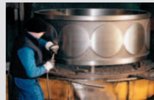
Tambour de cuisson de crêpes Ø1600mm - 900 kg Cooking drum for pancakes Ø1600mm - 900 kg
